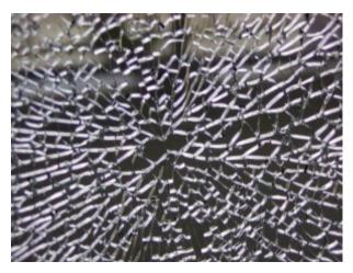
When tempered glass is broken (as shown above), it shatters into thousands of tiny pebbles, practically eliminating the danger of human injury caused by sharp edges and flying shards of glass.
